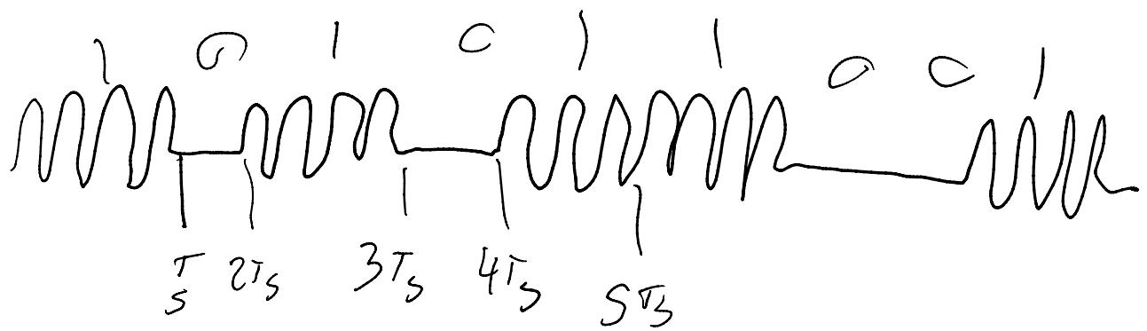
On-off keying - very natural, useful when TX mechanism has very high freq.
