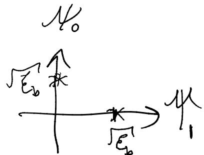
$$s_1 = (\sqrt{E_b}, 0), \quad s_0 = (0, \sqrt{E_b}) \text{ in this basis}$$
