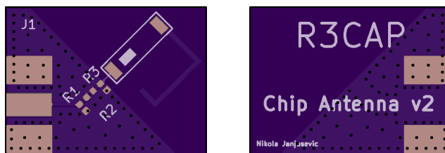
Figure 3: Render of antenna prototype boards, frontside left, backside right. The PCB has four layers (to simulate the four layer environment of the final board) and has space for a pi-matching circuit and chip-antenna.
