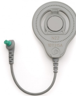
Fig. 2: The external component for a Nucleus Freedom, from Cochlear’s online store.
